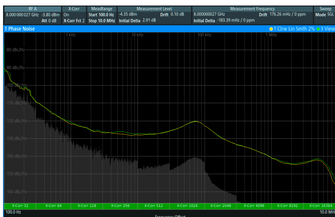
Phase noise measurement with the R&S®FSW3-KM129 option with cross-correlation. The yellow trace shows the measurement with amplitude noise rejection; the green trace without amplitude noise suppression; the grey area shows the cross-correlation gain.
