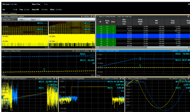
Multichannel approach: monitoring changes over time of the output signal of a radar jammer (blue traces) in direct relation to the radar input signal (yellow traces).
