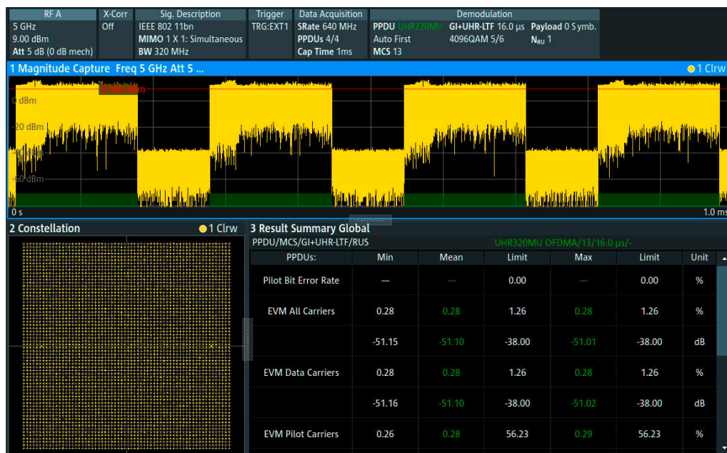
Analysis of a 4096QAM modulated 320 MHz wide IEEE 802.11bn signal
